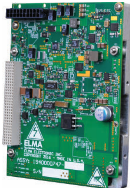
Elma Electronic engineers have designed their own CompactPCI small-form-factor embedded power modules to support the company’s line of small rugged embedded computers.
