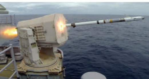
The Rolling Airframe Missile (RAM) Block 2, shown above, homes-in on its targets with infrared sensors.
