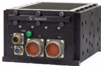
Falcon-Strike is a C5ISR small form factor, high performance multi-mission computer fielded for fixed and rotary wing missions as well as ground-vehicle counter-UAV applications.
